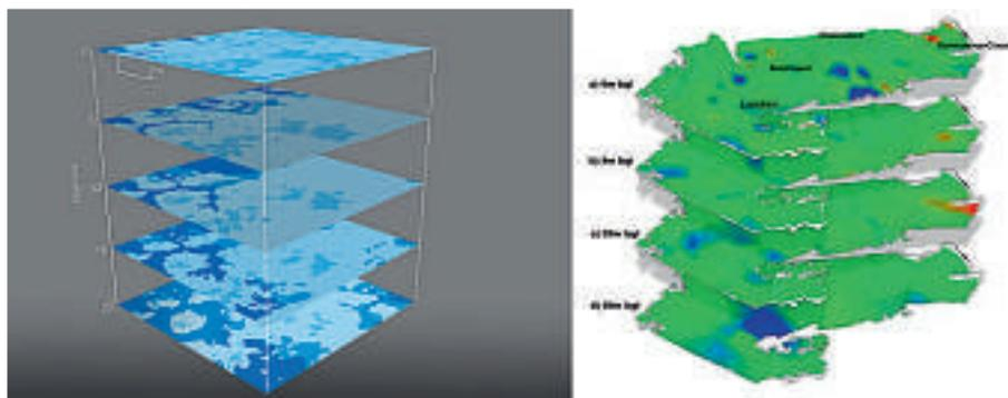
Fig.3: Left: Example of variation in Shrink-swell potential at different depths. Right: 3D volume change potential of the London Clay
