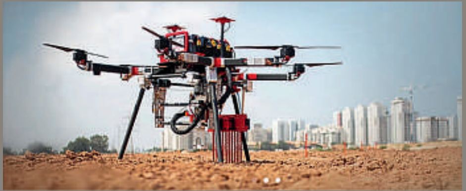
As well site surveying, drones are already being used to speed otherwise time-consuming tasks. Here, Civdrone's robotic system inserts 'smart' pegs into the ground that subsequently provide data to construction teams via a smartphone app. Photo: Civdrone
