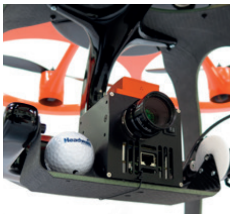
As UAVs get smaller and lighter, so too must the payloads they carry. Headwall's Nano-Hyperspec contains a very small, light hyperspectral sensor with embedded data storage and directly attached GPS
