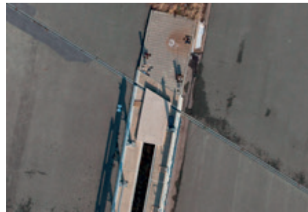
A ground control point in situ and at 1 cm/px resolution
