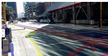
being used by utilities, contractors and asset managers all around the world. The **3D Augmented Reality** view is making the task of spatially locating and identifying underground assets considerably easier, and also enabling in-field capture and maintenance of asset data. [www.augview.net](http://www.augview.net)
