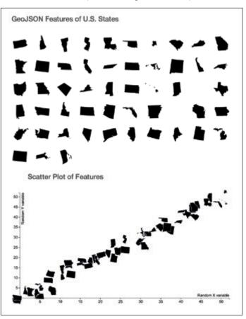
d3.geo.exploder enables you to move and resize features to other shapes, such as a scatter plot
