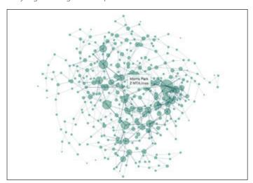
A directed graph of the New York Metro created by analysing the Google Transit specification for MTA using JSNetworkX and D3
