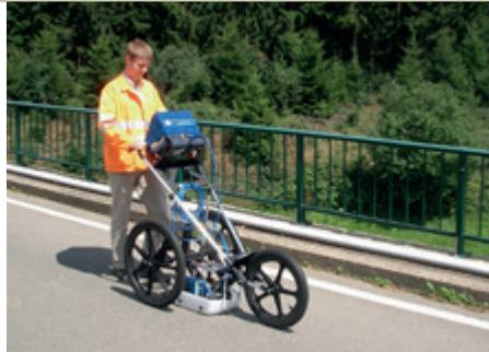
BridgeScan is tailored for bridge condition assessment, using a non-destructive method of evaluating bridge deck thickness, the system can obtain reliable thickness measurements in minutes, eliminating the need to core. [www.geophysical.com](http://www.geophysical.com)
