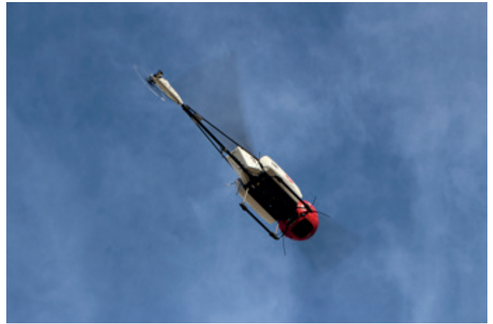
Flying-Cam 3.0 SARAH E, fully electric unmanned helicopter
