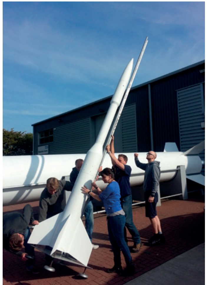
The Starchaser Tempest Rocket being readied for launch in Capesthorne Hall, UK. It has a small air quality sensor developed by the University of Leicester and Bluesky mounted in its nose cone
