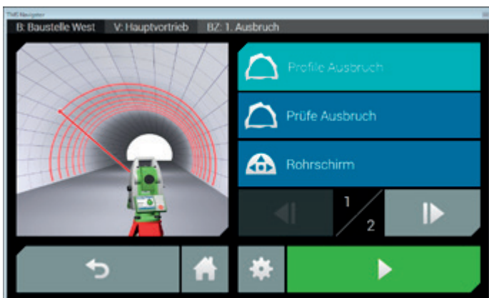
The 'Profiles excavation' measuring task
