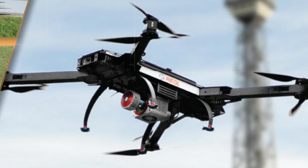
The RiCOPTER: First fully integrated LiDAR system solution
