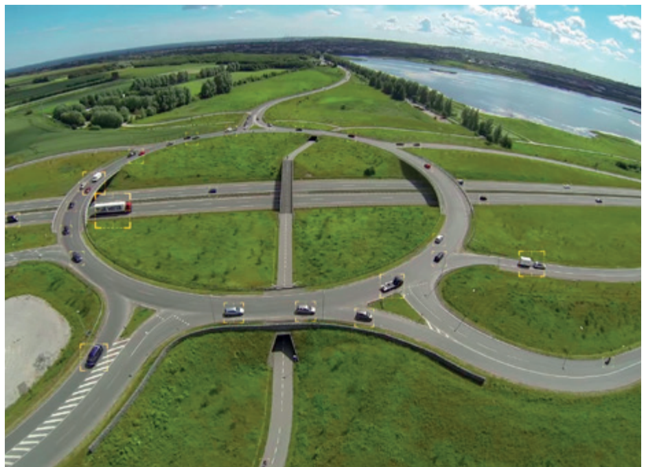
Beta version of software automatically counting traffic at a large roundabout north of Aarhus, Denmark. The software detects, marks and follows every vehicle entering and exiting the roundabout
