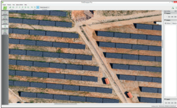
370 still images were processed in Pix4Dmapper Pro to create a georeferenced true orthomosaic of the PV field with 3cm GSD accuracy
