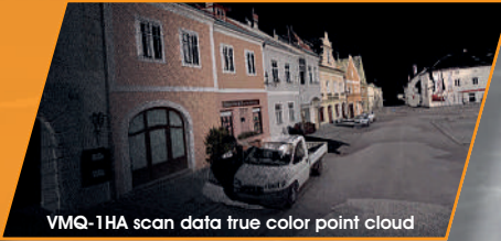
Infrastructure Mapping (VMX-1HA scan data acquired in a single pass)
