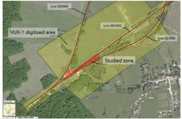
The typical complexity of railway mapping: parallel tracks, turnout/switch section, infrastructure elements (bridge, tunnel entry)
