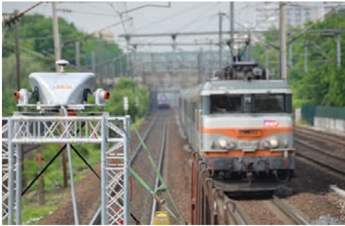
The RIEGL VMX-450 mobile scanning system mounted on an SNCF measuring train
