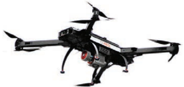
Delair Tech DT26X equipped with RIEGL VUX-1 scanning system
