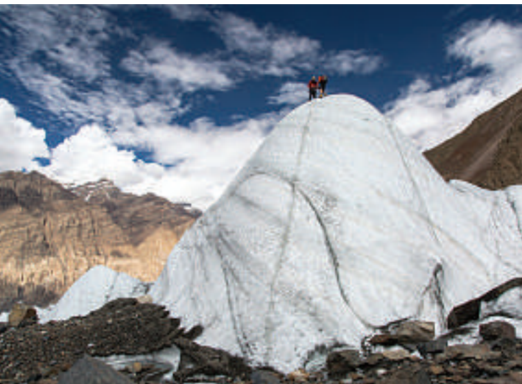
Sergiu Jiduc and Mathew Farrell install a measurement point atop a glacial mound. Though difficult to access, the high points provided good, recoverable locations for measurements. (© Tim Taylor, Karakoram Anomaly Project)
