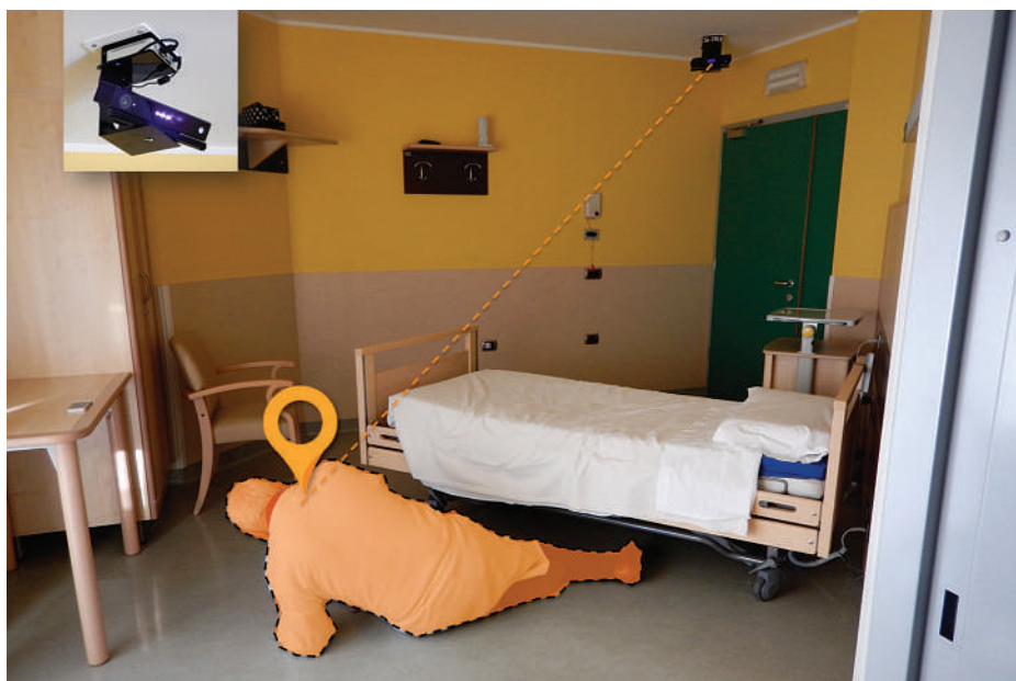
Detecting a fall using a wall-mounted Microsoft Kinect
