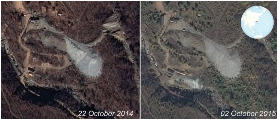
Figure 1. Pléiades images acquisition on 22 October 2014 (left) and 02 October 2015 (right) on the north portal. New spoil pile is visible on the bottom part of the image and main spoil pile has also increased (©CNES 2014 and 2015, Distribution Airbus DS)
