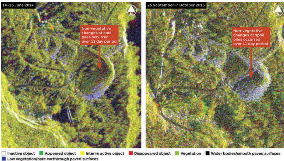
Figure 3. Punggye-ri, north portal: spoil piles change detection analysis using both optical and radar satellite imagery (©Cnes 2015, Distribution Airbus DS and ©DLR eV 2014-15 and ©Airbus DS Geo GmbH 2014-15/©2016 IHS)
