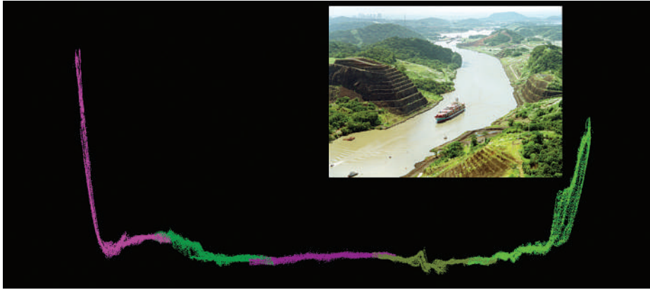
EM 3002 multi-beam bathymetry of Corte Culebra area. Image courtesy of Panama Canal Authority
