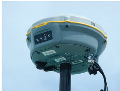
After working through the night a Trimble R8s GNSS receiver greets the sunrise on Carrie Bow Cay. The receiver operated continuously to produce 24-hour data sets needed to connect the island to control points on the mainland.
