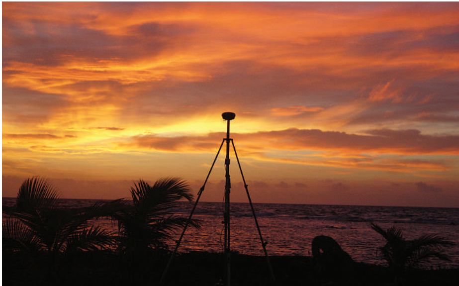
After working through the night a Trimble R8s GNSS receiver greets the sunrise on Carrie Bow Cay. The receiver operated continuously to produce 24-hour data sets needed to connect the island to control points on the mainland.
