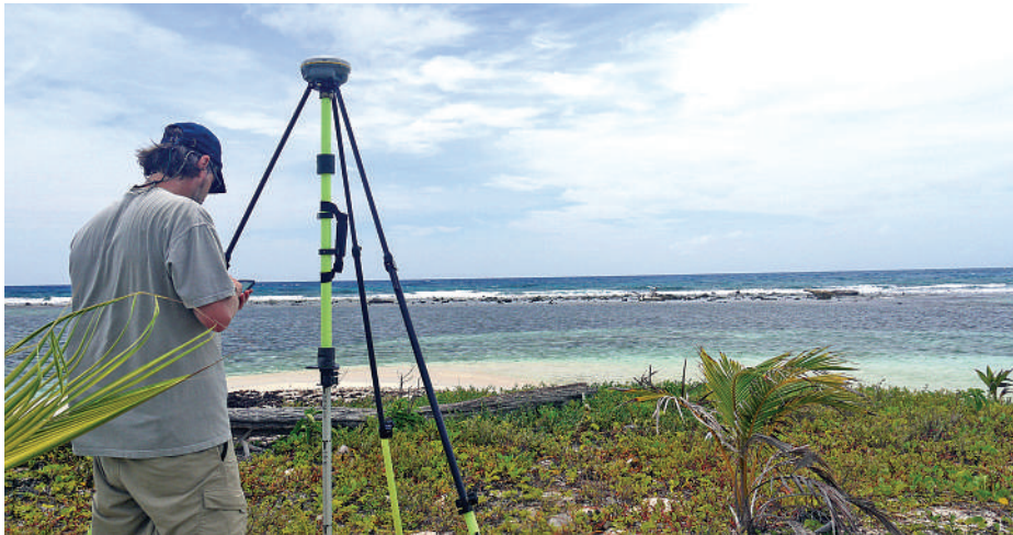
Set up at benchmark point CBC-South, Tim Smith uses an app on his smartphone to operate the Trimble R8s GNSS receiver. The receiver stored data internally for subsequent download and processing.
