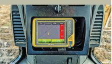
modelling to give the driver a view of the machine's cutting edge in relation to the final plans. This means operators are not relying on human judgement, which has a huge impact on the productivity, safety, cost and waste produced when working. www.topconpositioning.com/en-gb
