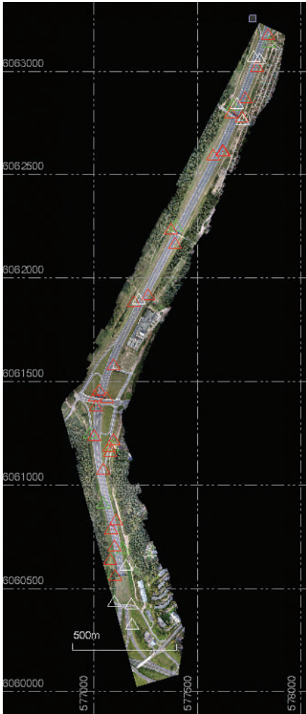
Combined images illustrate the extents of the project. Coloured triangles indicate ground truth points used to control and check the work
