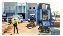
also layout or QA/QC (quality assurance/ quality control) with the BIM 360 Layout app." With the addition of the iX series, operators now have a choice of instruments in the Sokkia family with BIM 360 connectivity, including the SX total station series. www.sokkia.com.
