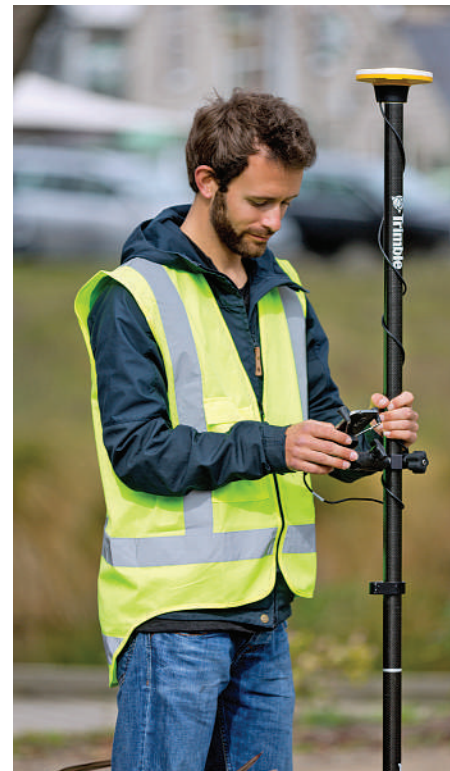
Catalyst, Trimble's latest GNSS-on-a-pole solution, is based on a subscription service that provides on-demand geo-location capabilities when combined with a small, plug-and-play digital antenna. Photo: Trimble
