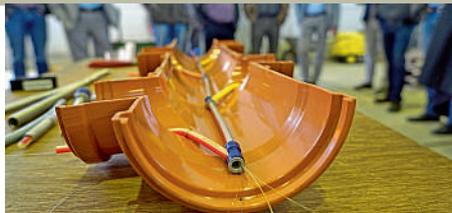
for infrastructure assets. The joint administration of control, broadband, fibre optics and energy cables in conjunction with networks in other sectors, such as sewer networks, has been realised by implementing a dedicated cable module. Here the routing of lines is possible through the conduits of the sewer sections in the sewer module. [www.barthauer.de](http://www.barthauer.de)
