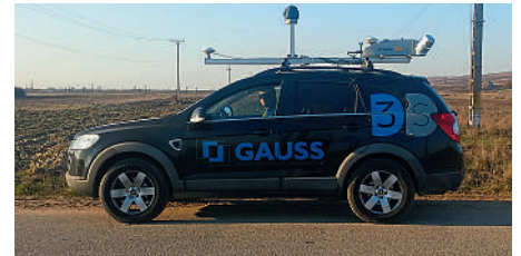
Gauss used a Trimble MX2 mobile mapping system to capture georeferenced scans and images at the Timisoara airport. They also use the system to survey highways and utility corridors
