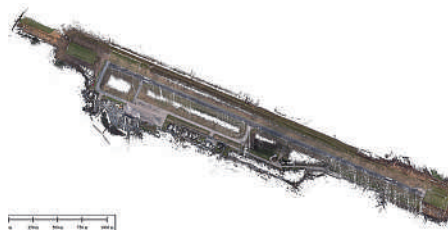
A high-level view of the 3D point cloud for the Timisoara airport. Surveyors needed roughly four hours to capture the information for the airfield and terminal areas
