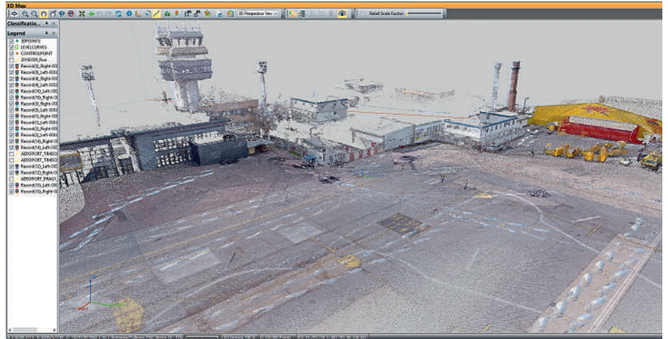
Scanning data from the mobile mapping system at the TVIA terminal area. The system used LiDAR and imagery to produce detailed database of airport assets
