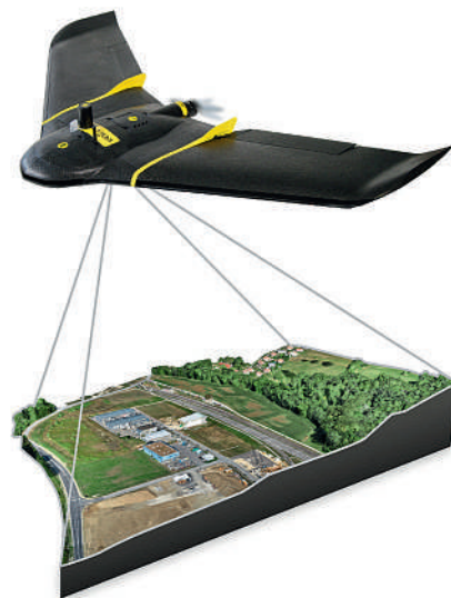
The eBee Plus suits a wide range of applications — from cadastral land surveying to quarry and mine mapping, land management, environmental and humanitarian projects. Image: senseFly
