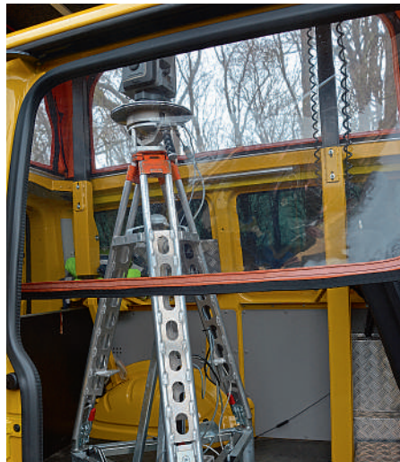
A total station installed in the survey vehicles. Custom-built tripods provide stable mounts and the ability to extend and retract as needed.
