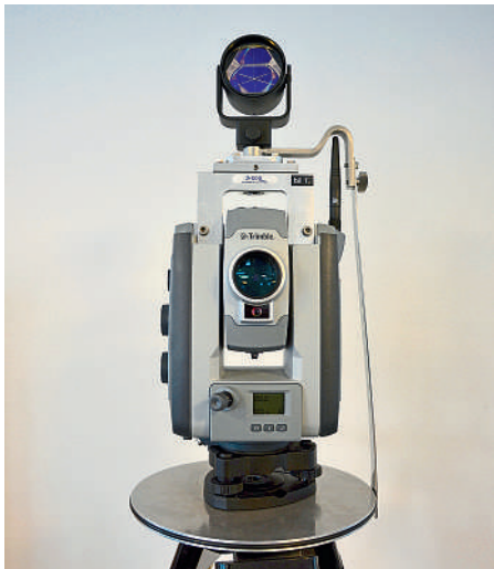
A total station and top-mounted prism assembly for reciprocal measurements. The prism rides in a rotatable bearing to provide stable orientation while the total station turns beneath it
