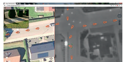
The bright white spots indicate heat loss. Using panoramic imagery can help determine if it is an issue that needs on-site inspection
