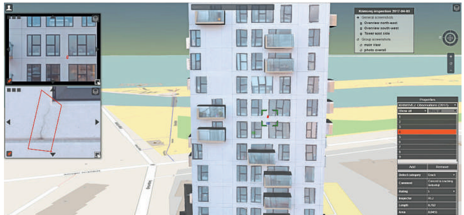
3D model with red marking at the location of the observation. The left side shows an overview and the close-up image shows detail; the right side shows a limited range of properties of the observation.
