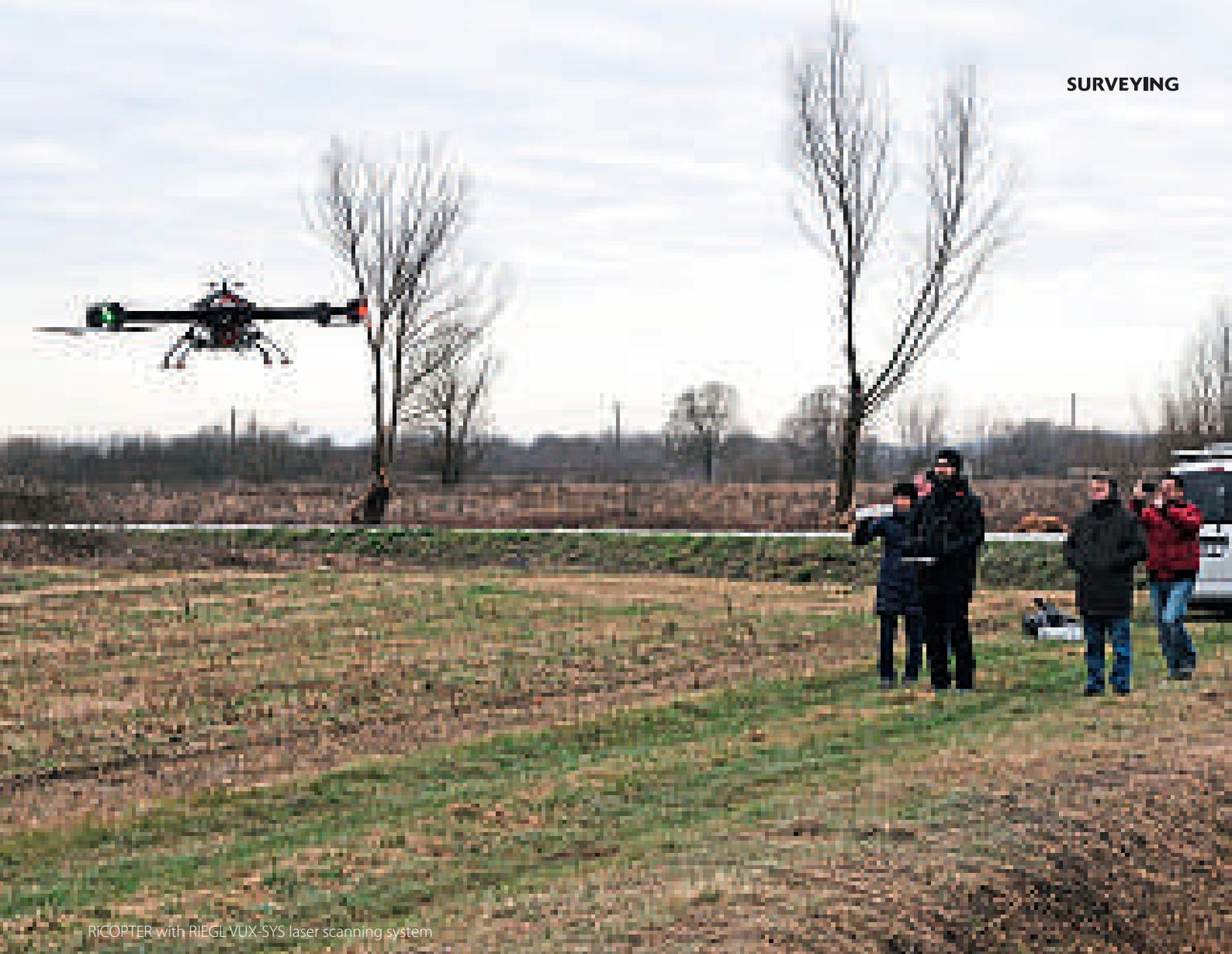
RICOPTER with RIEGL VUX-SYS laser scanning system
