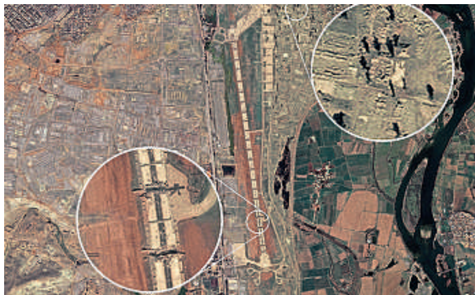
Figure 2. Deimos-2 image of Mosul's Airport: the airport runway was destroyed and infrastructures damaged. Upper zoom in: razed building; lower zoom in: rubble and trenches at runway. Image captured on February 19 2017
