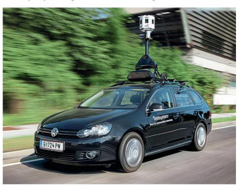
The UltraCam Mustang vehicle-based mobile mapping system represents a proven, state-of-the-art system for capturing street-level georeferenced panoramic imagery and 3D data
