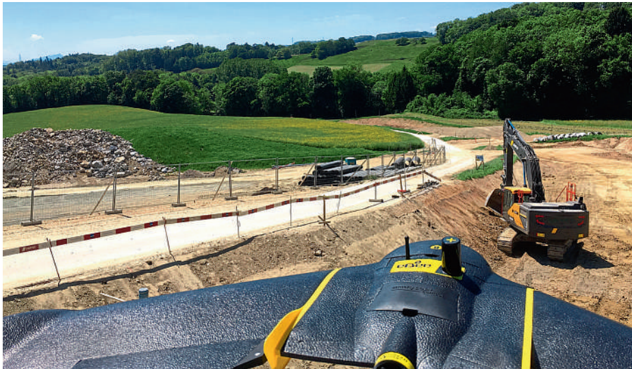
An eBee Plus UAV flying over a linear site
