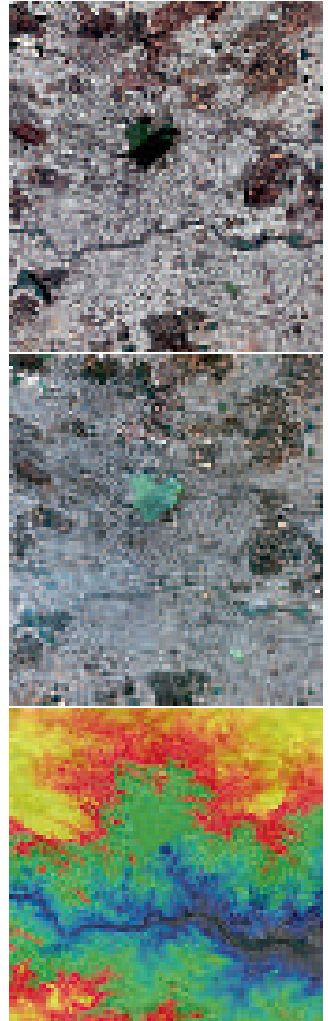
Figure 4. (l-r) Deimos-2 stereo product acquired over Hyderabad on January 5 2017 at 11:06 UTC and 11:08 UTC, together with derived DEM
