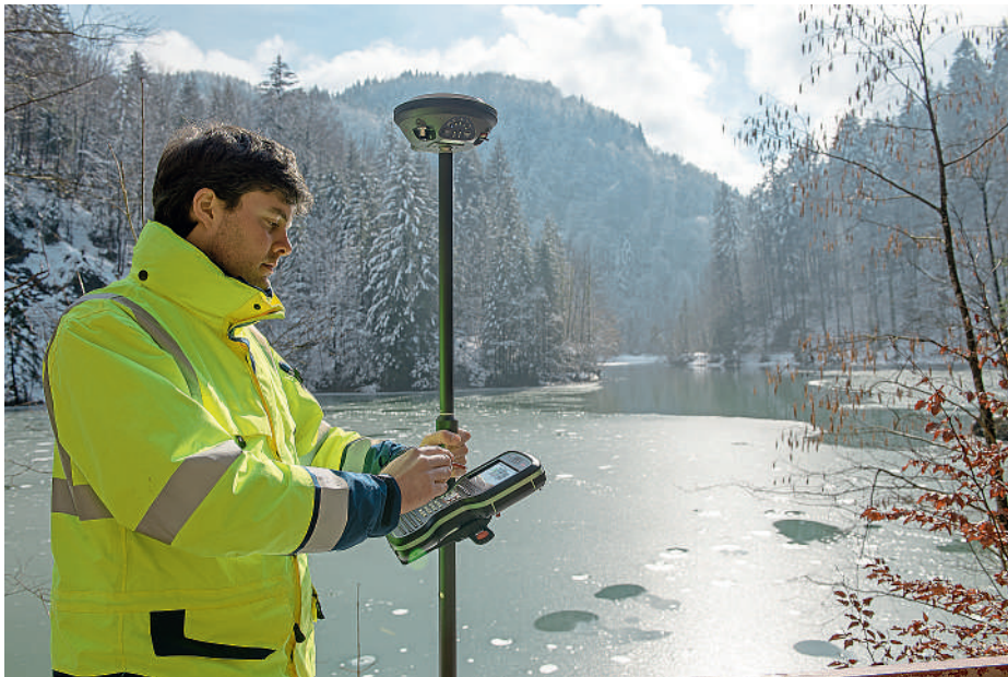
The most precise surveying instruments offer functionality where the receiver automatically switches between the best possible reference link, such as the GS16 with SmartLink
