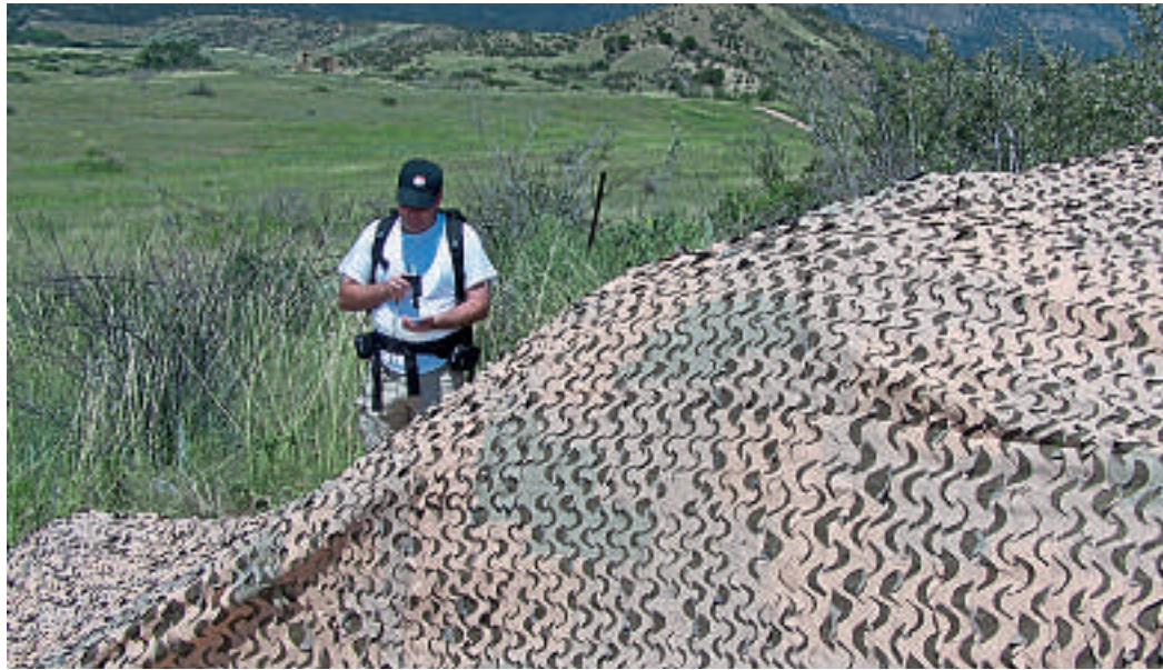
Calibrating ASD's FieldSpec 4 for field collection of camouflage spectral signatures
