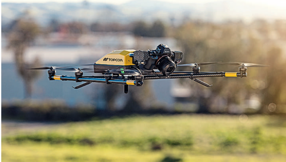
The Falcon 8+ UAV Topcon edition carries both GNSS technology and a video camera
