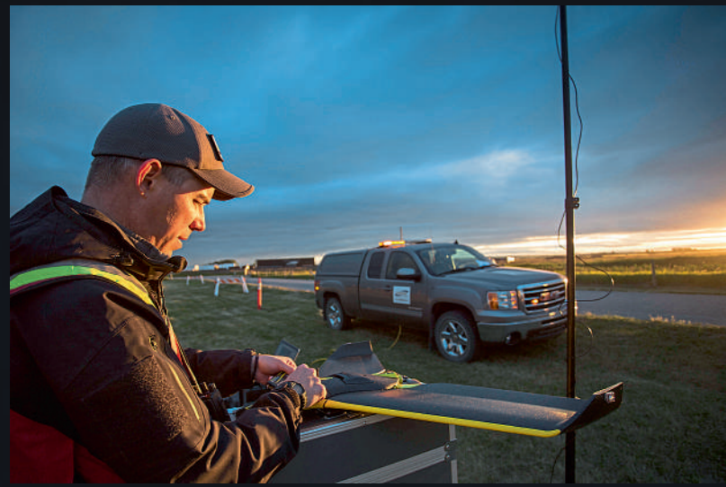
IN-FLIGHT Data's BVLOS UAS Operations trial uses a senseFly eBee and eBee Plus to conduct flights across Canada © Droto – Marcel Vajdik
