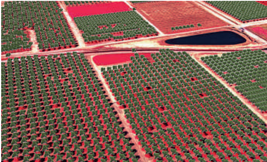
An overview of the identified tree locations using CNN, overlapped on a false-colour composite of the UAV's mosaic
