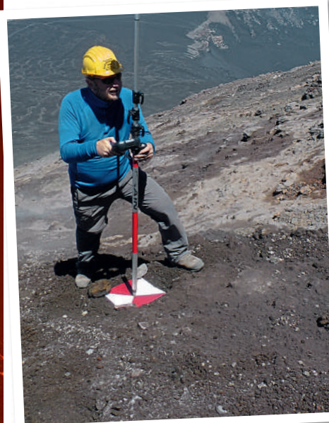
Juraj Papčo measures a position for topographic mapping high on Mount Etna. Measured points were compared with models created from aerial imagery
