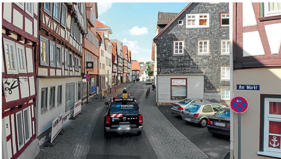
The mobile mapping system was mounted on the roof of a car, capturing 700,000 laser measurement points per second
