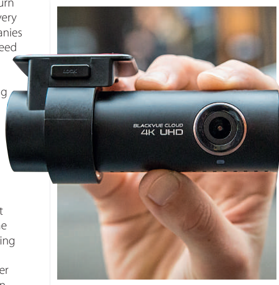
The Mapillary Dashcam is the world's first end-to-end encrypted dashcam built specifically for mapping purposes
