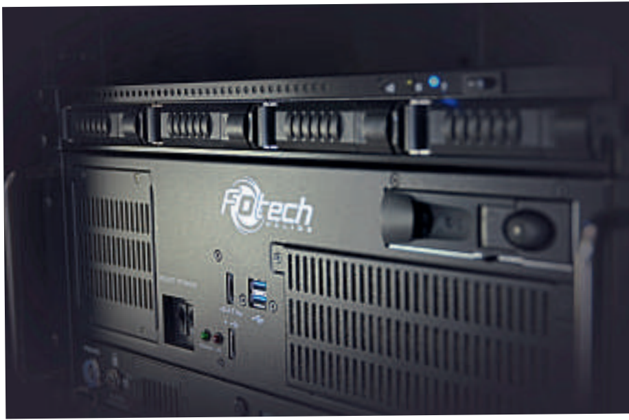
DAS 'interrogators' plug in to standard fibre optic cable networks, converting them into sophisticated acoustic sensors to monitor traffic flows
