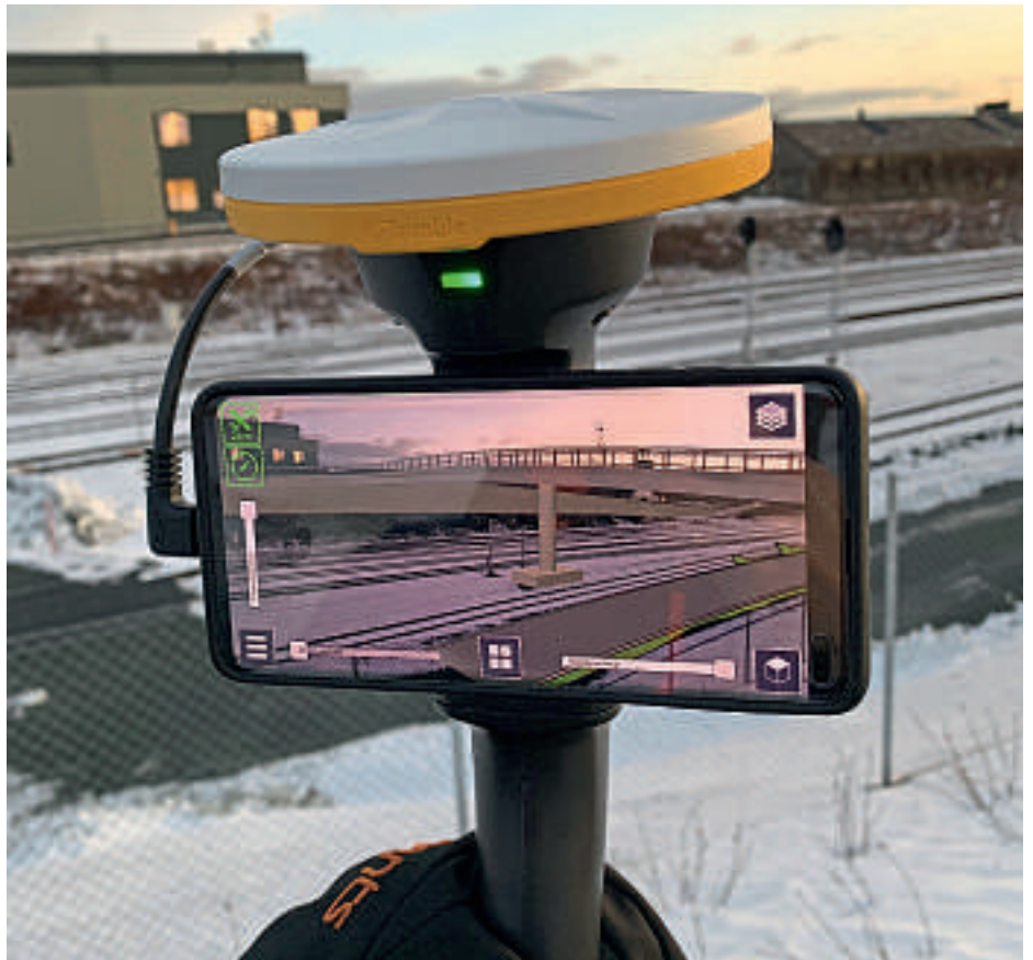
ViaNova deployed SiteVision on smartphones, with the companion Catalyst GPS system providing the precise position and orientation. Shown on the display are the proposed bridge model projected in real-time over the landscape
