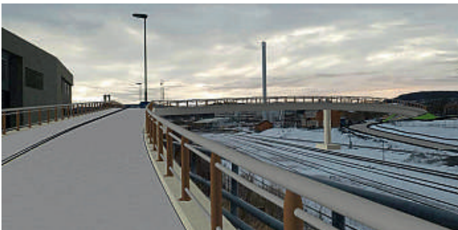
AR shows that the bridge access ramp passes behind the nearby residential structure. ViaNova used this discovery to inform design changes
