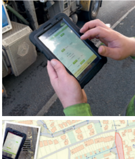
The 'Gully SMART' system uses OS MasterMap to map and monitor drainage networks and other local authority assets
