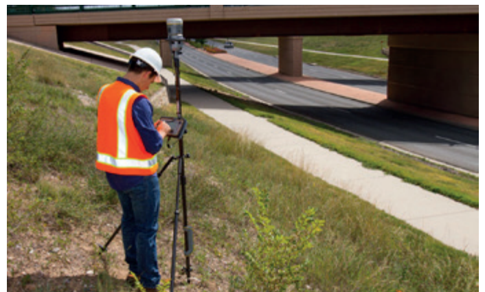
Using a Trimble V10 imaging rover with Trimble R10 GNSS receiver, a technician captures georeferenced panoramic images for bridge inspection. The system enables capture of comprehensive information while working a safe distance from traffic or other hazards
