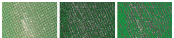
Ecognition Essentials is used to check the percentages of plant and soil as the potato crop grows
