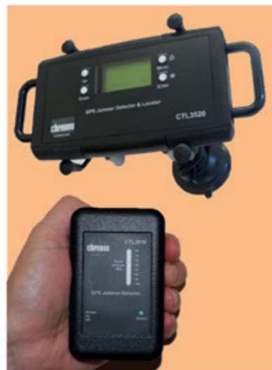
(Left): The Exelis Signal Sentry 1000 user interface supports timely and effective actionable intelligence in GPS denied and contested environments (Image: Exelis Inc.), while (Right) handheld units from Chronos Technology will detect and locate jamming signals in the GPS –L1 band (Photo: Chronos Technology)
