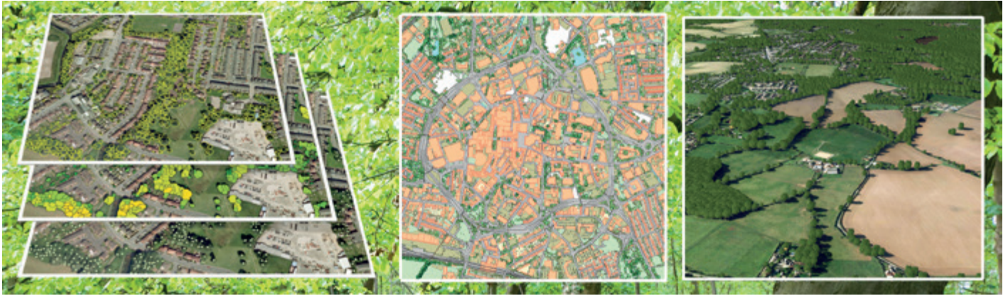
Pictured from left to right: NTM's three vector map layers; tree cover aligned with mapping, and oblique aerial photography to aid the capture of height points
