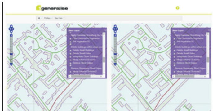
The 1Generalise dual viewer allows the user to compare any pair of intermediate states in the process. This is useful for tuning parameters.
